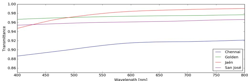
Fig. 5. Hemispherical transmittance in the visible range of coupon 3, referenced to the transmittance of coupon 0, in Chennai, Golden, Jaén and San José at the end of the data collection period. The spectra were measured with different spectrophotometers at each site.
